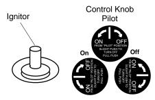
Figure 22 - Ignitor and Control Knob
